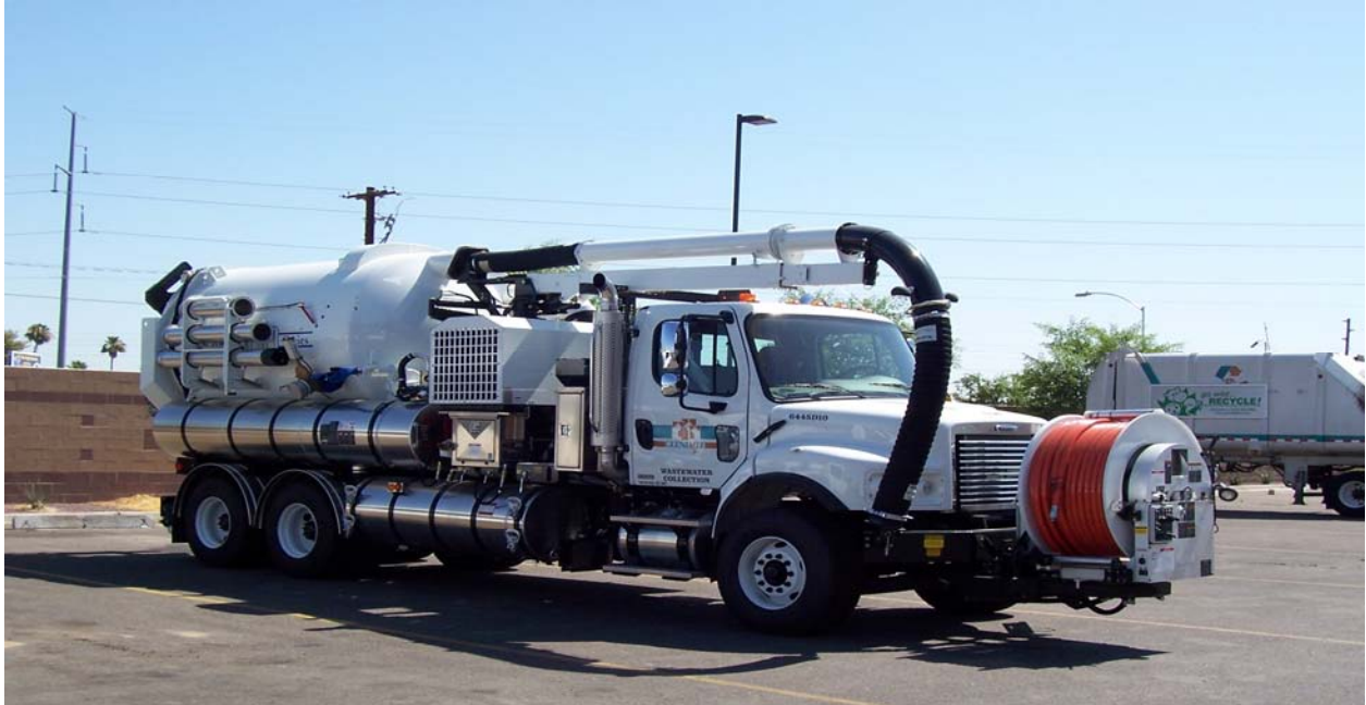
Waste Water Truck
